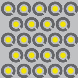
A schematic representation of the 23 SPADs placed on a hexagonal grid.
